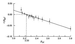
**Fig. 4.** The function  $f(D_{el})$  as described in the text is the average of data taken from 20 scans, and is based on 15 different values of  $D_{el}$  and 9 reflectivity thresholds (for a total of  $9 \times 15 \times 20 = 2700$ dimensions). Averages and standard deviations, indicated by the error bars, are plotted. The leastsquares linear regression is shown and has a horizontal intercept ( $D_{\rm el} = d_{\rm el}$ ) of 2.22.
