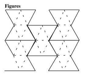
1 Viscoelastic honeycomb structure. It exhibits a decreasing Poisson's ratio provided that the solid lines represent elastic ligaments and dashed lines represent viscoelastic ligaments which relax with time to zero stiffness.
