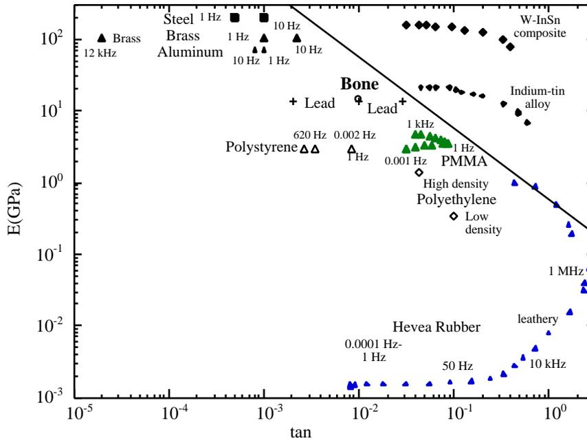
Fig. 2 Stiffness-loss map for some materials. Temperature is near room temperature. Adapted from Lakes (1998). Data are replotted from several sources, including Brodt, et al. (1995) for indium-tin alloy.
