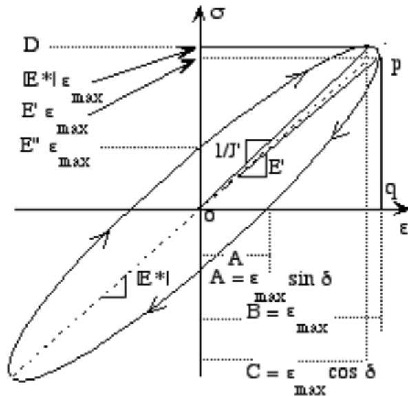
Fig. 1 Stress vs. strain for a linearly viscoelastic material under oscillatory loading, after Lakes (1998). Illustration of slopes and intercepts. A material with a rather large value of  $\tan \delta = 0.4$  is shown for illustration. The material could be a viscoelastic rubber.
